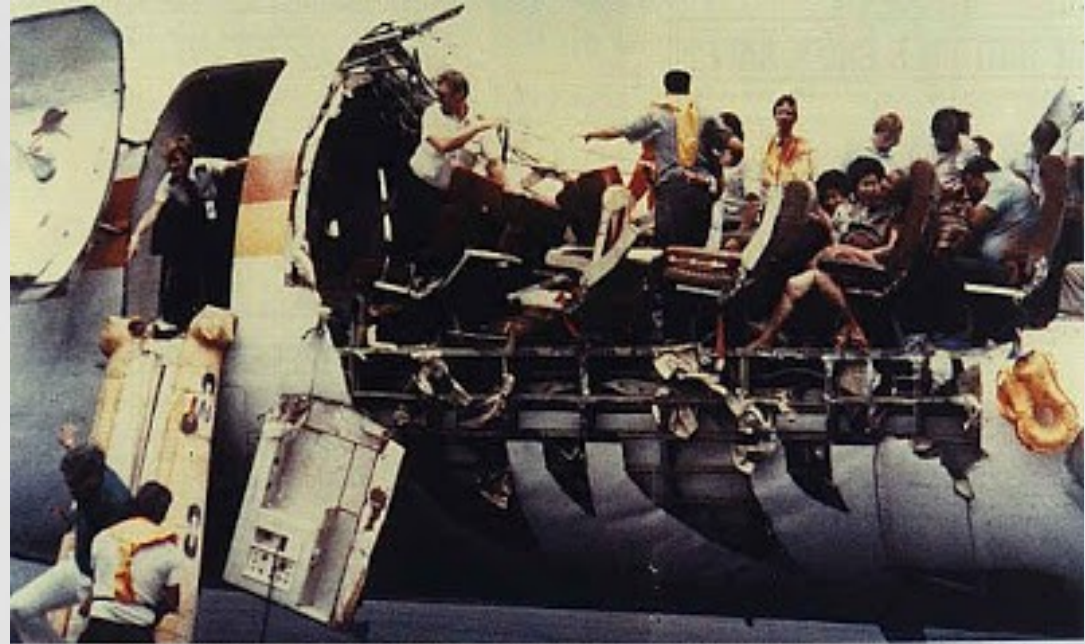
4-28-1988 After 89,090 flight cycles on a 737-200, metal fatigue lets the top go in flight.
